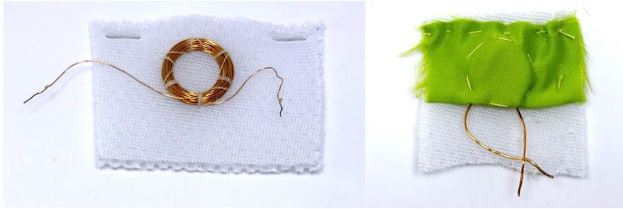
*Figure 6. Electromagnet (Left: Without magnet. Right With magnet)*
