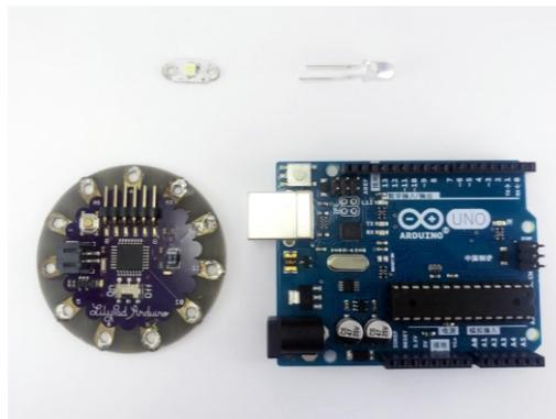
*Fig 1. Top Left: Sewable LED (Electro-fashion by Kitronic), Top right: 5mm LED, Bottom Left: LilyPad Arduino microcontroller, Bottom Right: Arduino Uno microcontroller*
