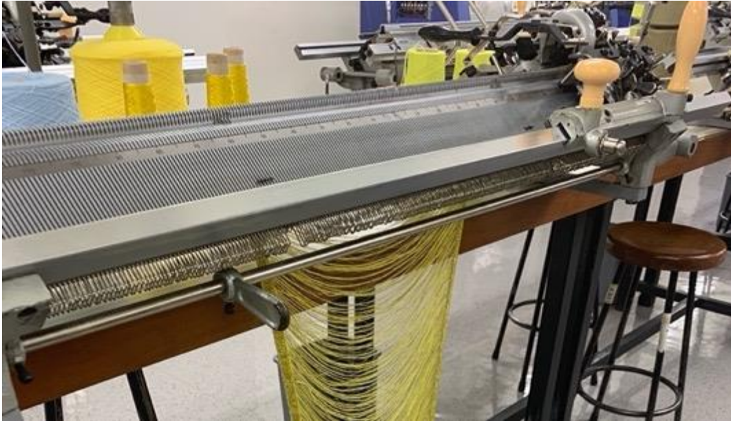
Figure 2. Wealmart knitting machine
