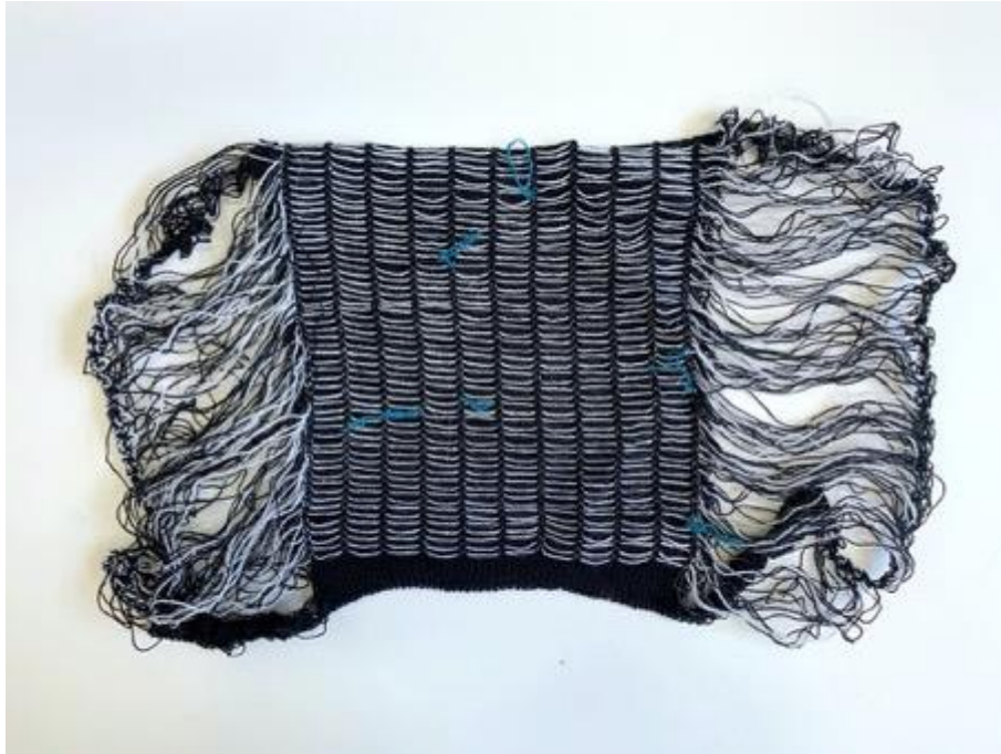
Figure 8. POF knit sample with white support yarn. Breakages marked with blue yarn
