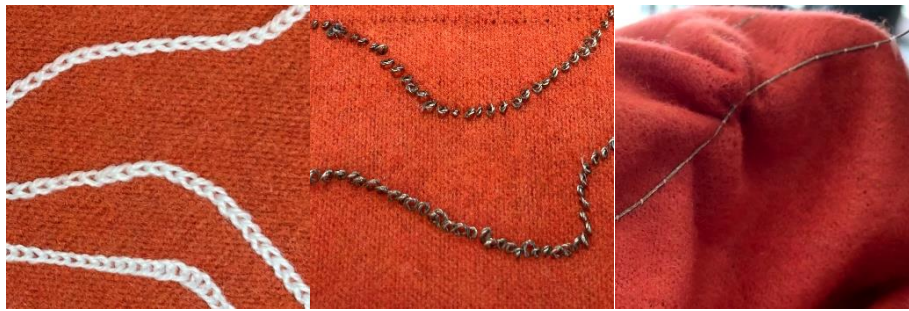
Fig. 1. Chainstitch (Left), Moss stitch (Middle), Lockstitch (Right)
