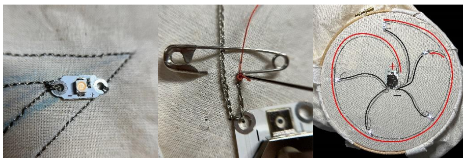
Fig. 3. LED stitched onto the circuitry (Left), Contrasting stitching (Middle), Parallel e-textiles circuit (Right)
