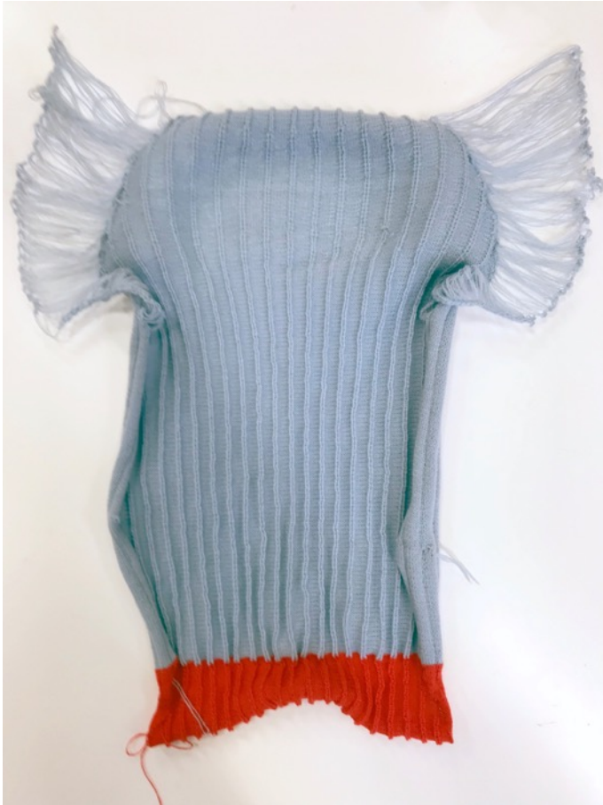
Figure 11. Knitted POF raglan jumper front piece (Pre-bundling)
